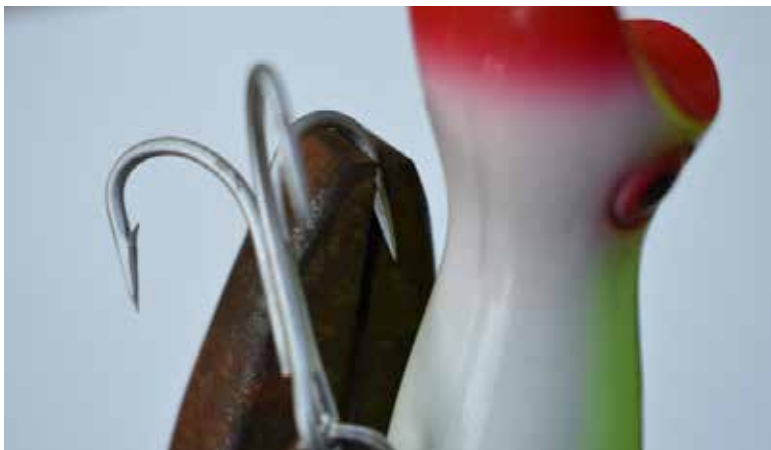
Crush barbs with Lineman's pliers. Angle the pincers to avoid damaging the hook point.
